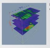
It is possible to locate each reflector occurrence coordinate in the testing object.
